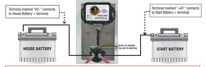
RED indicates original battery wiring. Do not change these as long as the House and Start circuits are independent of each other. Any Selector Switch should NOT be in the "Combine Battery position. E-Trak Marine does this function automatically.
