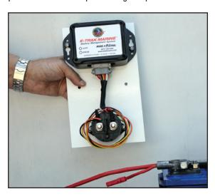
**STEP #3**Drill 3/32" holes for the mounting screws. Holes should be 3/8 to 1/4 inch deep. **DO NOT DRILL INTO OUTER HULL. CHECK TWICE BEFORE DRILLING.**
